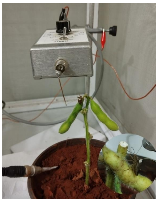
Figure 1. Monitoring the feeding behavior of Euschistus heros on soybean pods using Electropenetrography (EPG).
