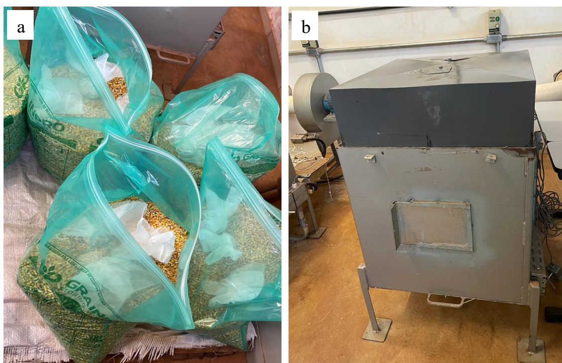
Fig. S1 Illustrative image of the hermetic packaging (a) and experimental silo (b) used for storing corn grains
