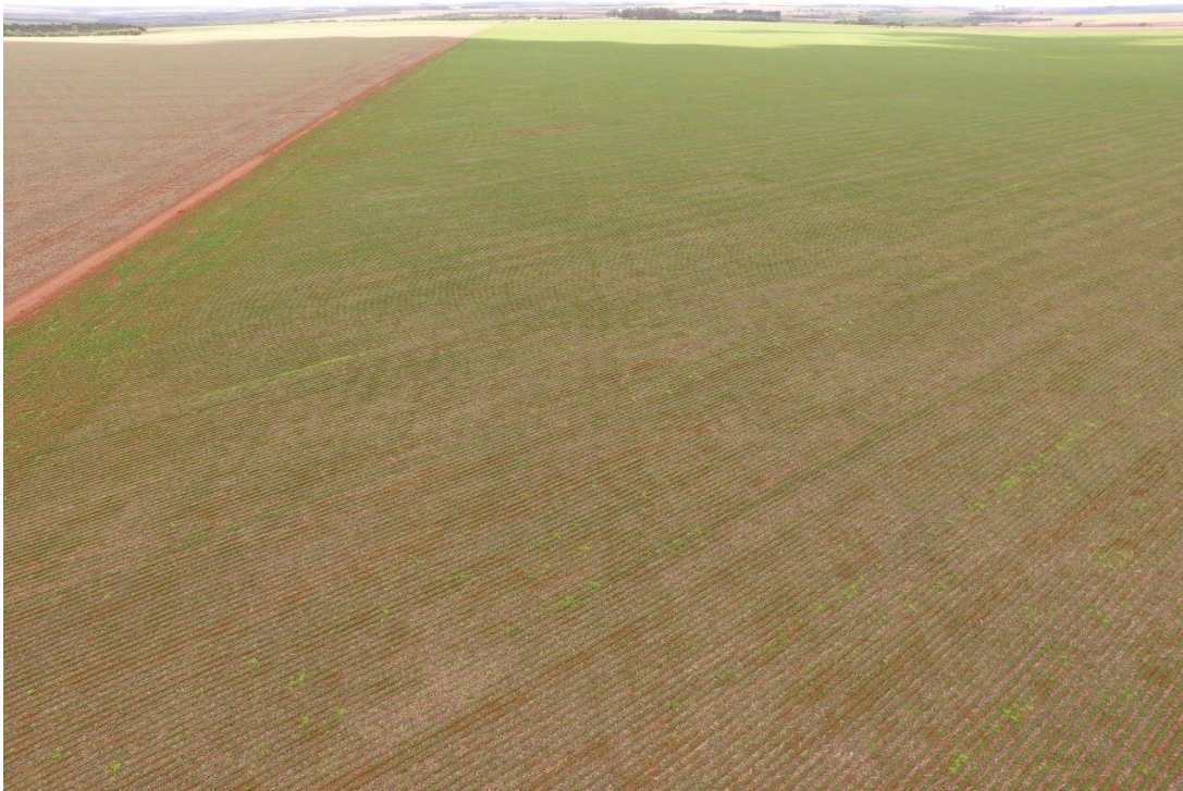
Figure 1 - Exploratory flight using a multirotor drone and an RGB sensor flying at 120 m high. Potential spots of plants infested with Heterodera glycines on soybean were identified by a trained researcher using orthomosaic images. A subsequent field visit was done to confirm the infestation.
